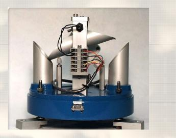
The **tipping bucket rain gauge** consists of a funnel that collects and channels the precipitation into a small seesawlike container. After a pre-set amount of precipitation falls, the lever tips, dumping the collected water and sending an electrical signal.
