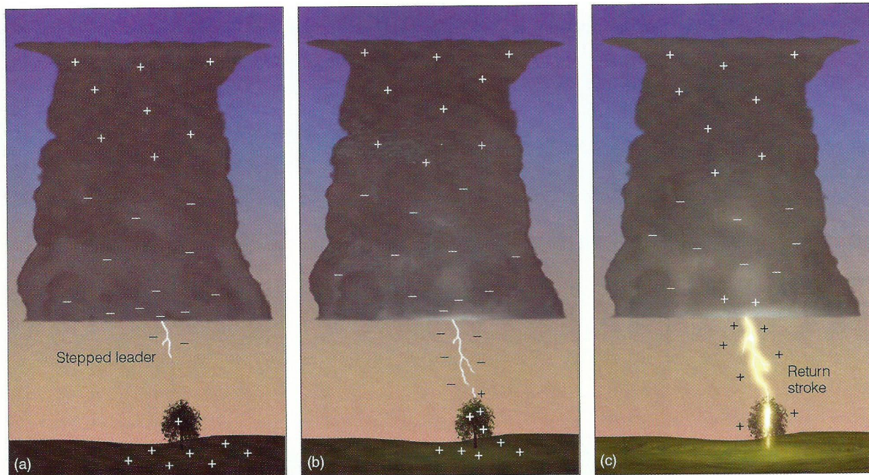
● Figure 10.28 The development of a lightning stroke. (a) When the negative charge near the bottom of the cloud becomes large enough to overcome the air's resistance, a flow of electrons—the stepped leader—rushes toward the earth. (b) As the electrons approach the ground, a region of positive charge moves up into the air through any conducting object, such as trees, buildings, and even humans. (c) When the downward flow of electrons meets the upward surge of positive charge, a strong electric current—a bright return stroke—carries positive charge upward into the cloud.
