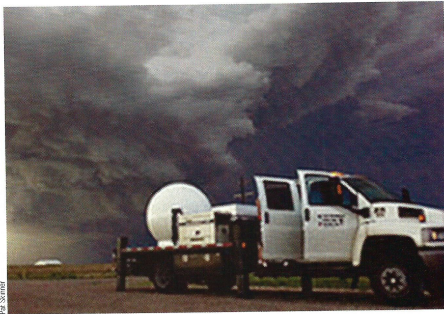
● Figure 10.56 Researchers from Texas Tech University set up a mobile Doppler radar unit near a supercell thunderstorm.
