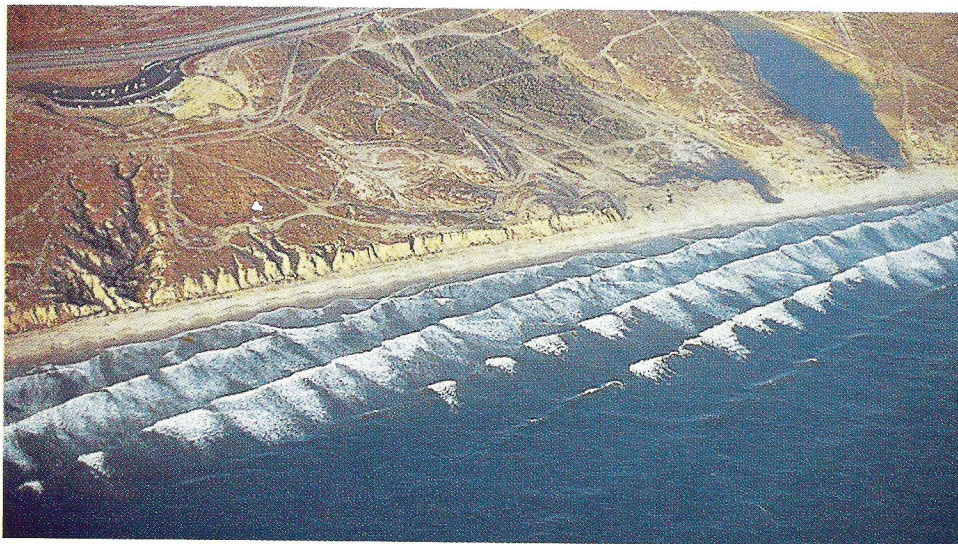
FIGURE 17.5 Waves obliquely approaching the shoreline and being refracted to be almost parallel to the shoreline. The white color shows the surf zone. Oceanside, California. (John S. Shelton.)
