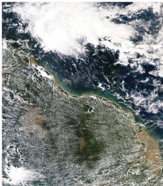
Figure 5.1 True color image of an Aqua scene from 20 November, 2000 at 1710 UTC, encompassing north-central South America, specifically Trinidad, Venezuela, Guyana, Suriname, French Guiana, and Brazil. This true color image is created by superimposing three bands: 0.65\ \mu\text{m} (Band 1 in red), 0.55\ \mu\text{m} (Band 4 in green), and 0.47\ \mu\text{m} (Band 3 in blue). Clouds are white but display a variety of textures and spatial scales. The land surfaces appear as green or brown depending on the amount of surface vegetation, while deep ocean appears as dark blue. Shallow coastal waters are light blue or brown in appearance
